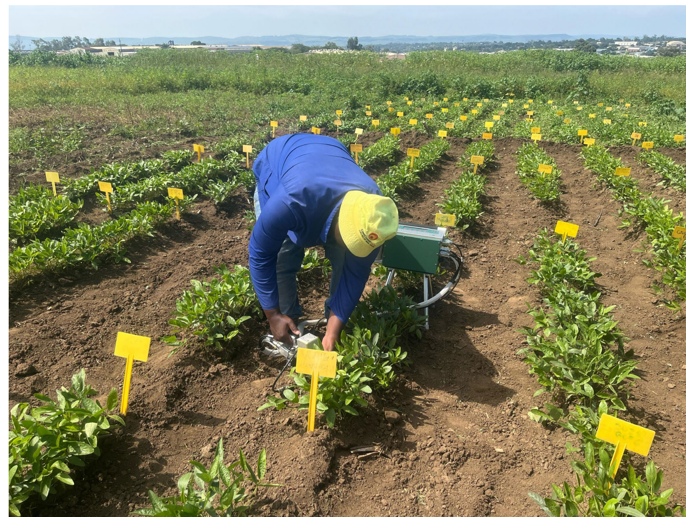
Figure 3: Measuring gas exchange and chlorophyll fluorescence parameters using Licor (LI-6400 XT)
