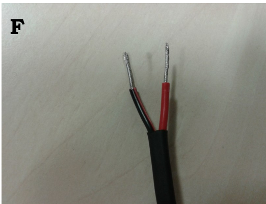
T-sense cable ends with pins removed and cable twisted
