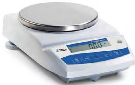
1. Make sure the balance is levelled. Use the two front feet of the balance for levelling until the air bubble is centred in the level indicator.
