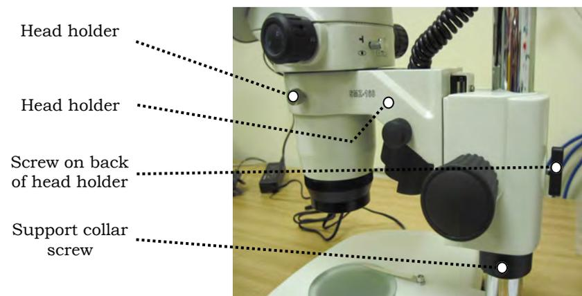
3. Looking through the eyepieces, move the head holder up or down until the specimen comes into focus. Tighten the head holder locking screw and do not let go of the head.
