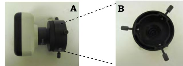
4. Place the camera assembly onto the microscope eyepiece (C) by attaching the Ø38 eyepiece adapter and tightening the three centring screws. Connect the USB power supply from the computer (or via the plug) to the adapter point (on the Moticam case). The light will flash and turn solid blue when the camera is ready.
